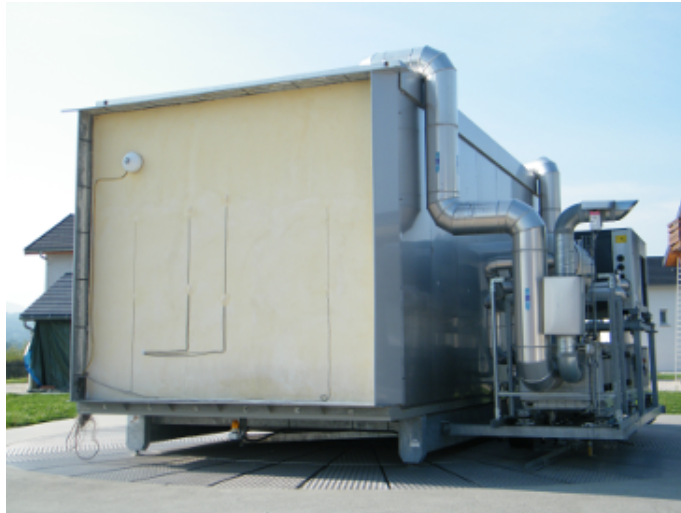
Figure 5: PASSSYS instrumented test cell
